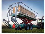
${f H}$ ydraulic platform is recommended for orchards with a row spacing wider than 3,5 m.
