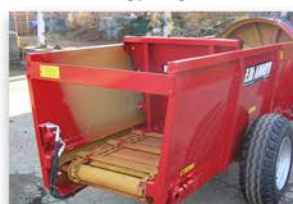
Sponda posteriore mobile ad avanzamento automatico Rear door advancing pushing manure to the turbine
