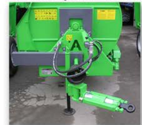
Timone sterzante meccanico Mechanical steering rudder to enter/exit easier in the row
